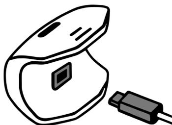
You will find the charging plug on the inside of the E-Unit. Insert your Micro USB cable to charge. If the button is blinking green, you have inserted your cable correctly and your Airofit is charging.
